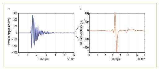
Fig. 4 Time trace measured by optical hydrophone, showing the pressure amplitude of a Doppler signal in the kPa amplitude range emitted by a linear array transducer (a). Typical photoacoustic pressure pulse in the single Pascals amplitude range (b).
