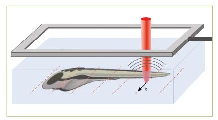
Fig. 5 Measurement principle of photoacoustic microscopy in reflection-mode. Zebrafish larva anesthetized in tricaine and embedded in agar (blue) are scanned by a focused laser beam (red) and the photoacoustic waves are detected by the optical hydrophone (gray).
