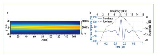
Fig. 3 Measured pressure field of a 10 MHz Panametrics V311 piezoelectric transducers (a). Pressure amplitude in far field and corresponding amplitude spectrum (b).
