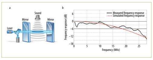
Fig. 2 Principle of operation of the optical sensor. The ultrasonic signal is detected optically by the change of the refractive index within a Fabry-Pérot etalon (a). Measured frequency response of the all-optical rigid sensor plotted as a solid black line and the simulated frequency response plotted as a dashed red line (b).
