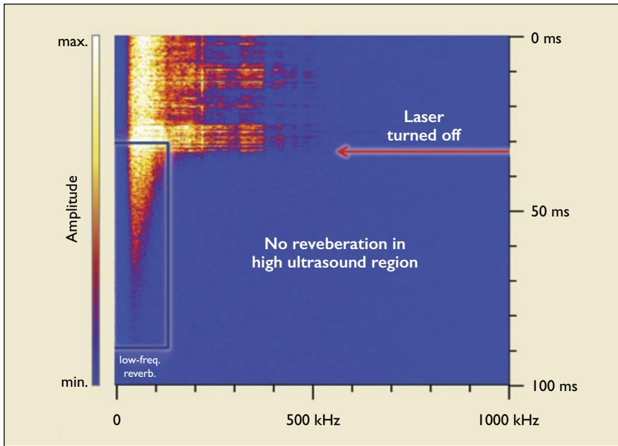
Figure 3. Typical acoustic 3D-spectrogram of PBF process (end sequence) captured by the Optical Microphone. Lack of reverberation in the high ultrasound regime enables superior resolution of process events.
