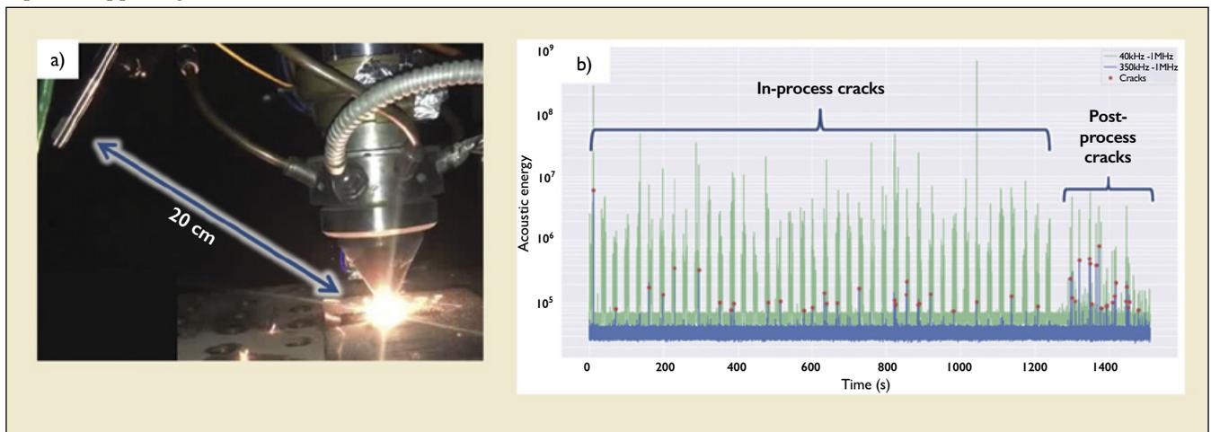
Figure 2. Typical measuring distance in an LMD process (2a). Ultrasound signals in the range of 350 kHz-1 MHz associated to cracks during and after a 20 min building process (2b).
