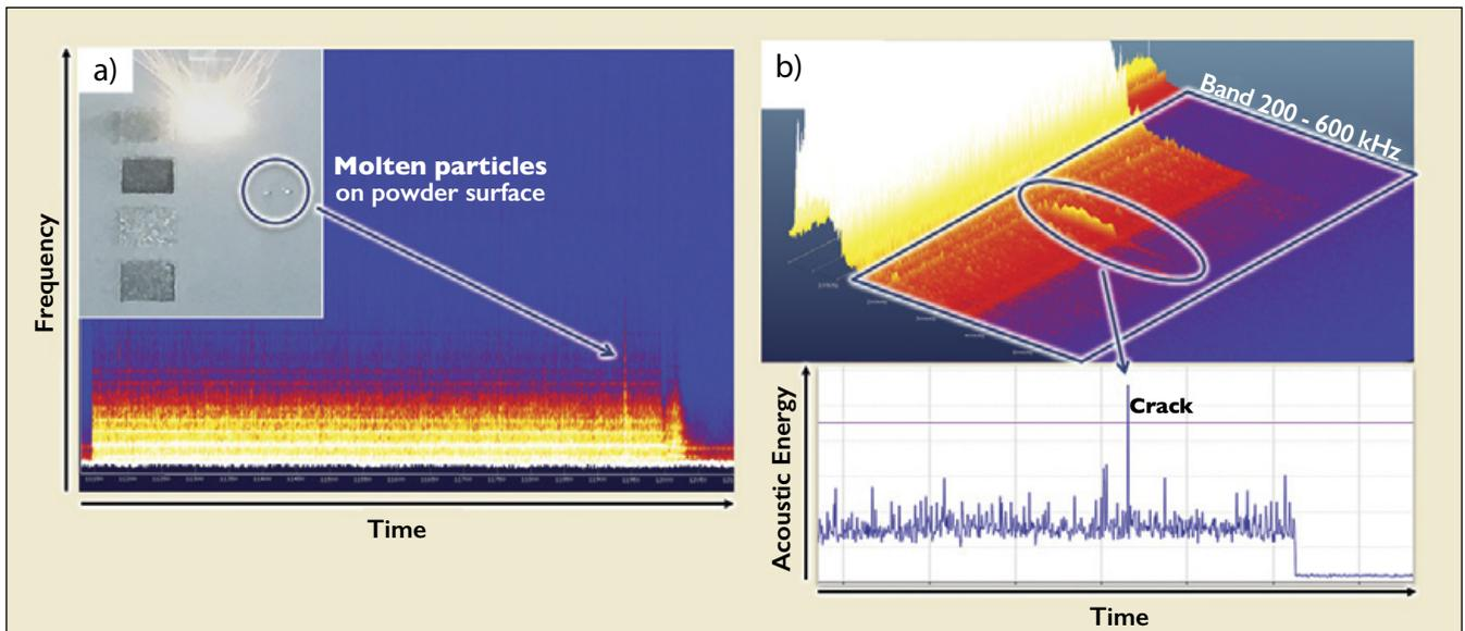
Figure 4. Two examples of short-term, broadband acoustic anomalies related to a) molten debris on the powder bed and b) cracking during the PBF process.
