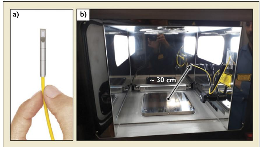
Figure 1. The fiber-coupled ultrasound sensor (a) within the PBF build chamber (b) at 30 cm measurement distance from the center of the build plate.
