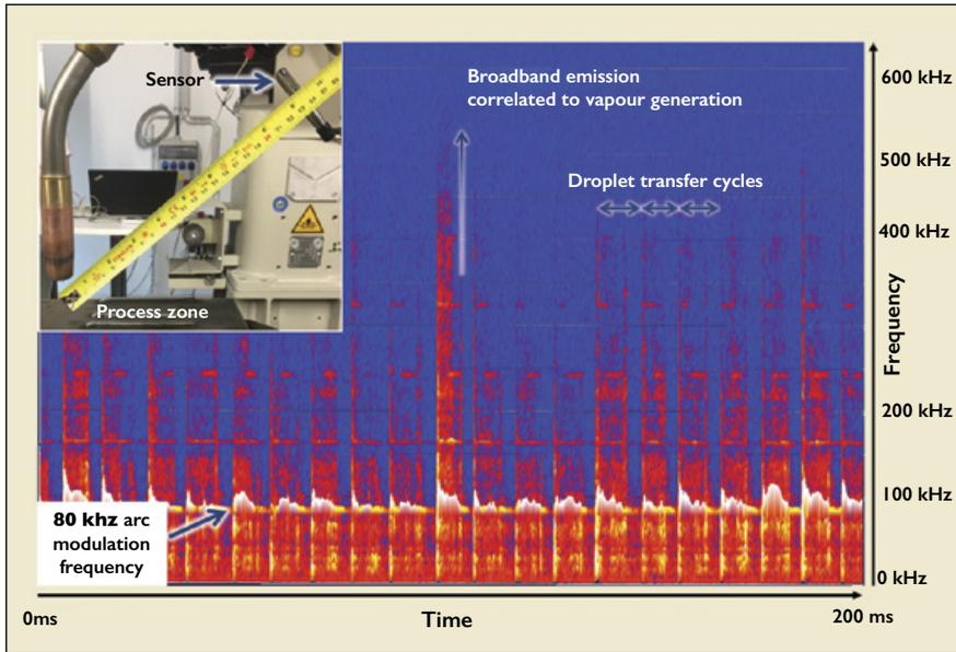
Figure 5. Positioning of the Optical Microphone in the Wire Arc AM process (inlay) and the corresponding acoustic signature of a 200 ms process section.
