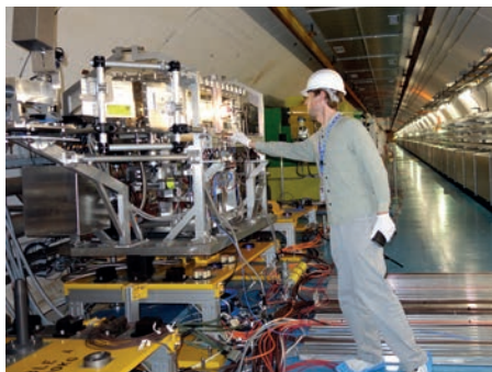
Figure 3 | Acoustic emission monitoring at CERN, where the robustness of different materials against proton-induced damage is being investigated. Figure courtesy of Daniel Deboy, XARION.
