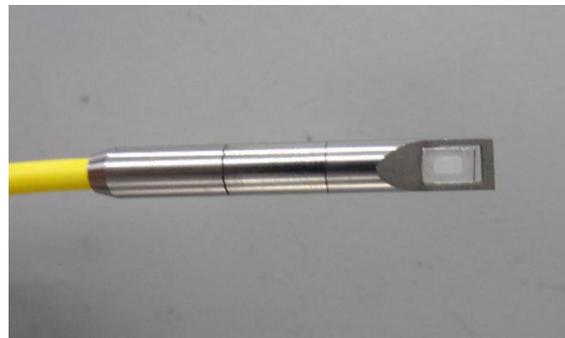
*Figure 1: Sensor head of the microphone*
