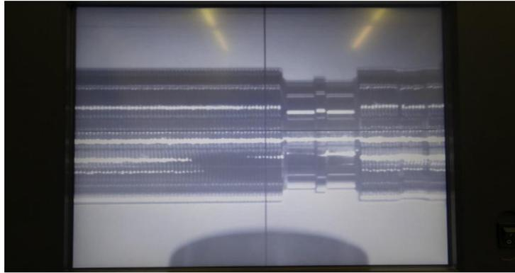
Figure 26: The display on the laser control panel, with the center of the crosshair pointing directly at the welding point
