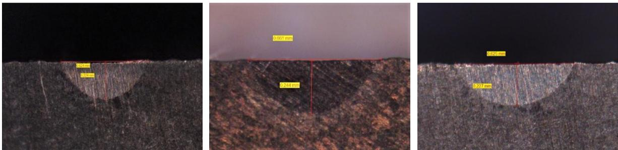
Figure 29: 3 weld seams from different cross sections of a weld seam at 280W laser process
