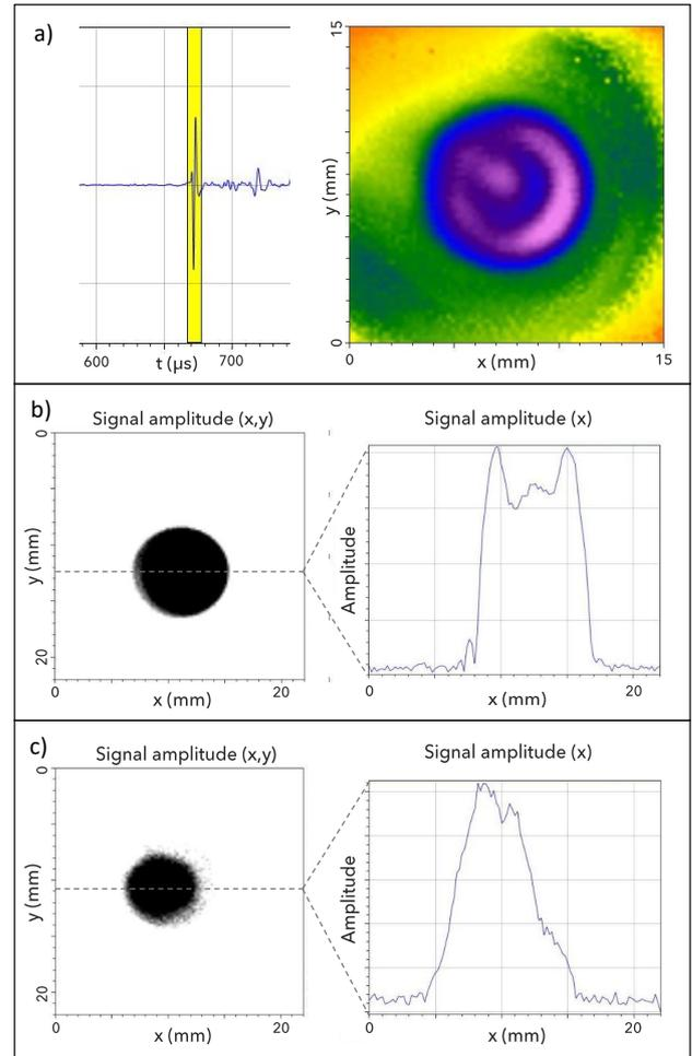
**Figure 3:** Results of the through-transmission measurements. (a) Typical time signal and C-scan of the spot weld. (b) Thresholded C-scan and line scan along x-axis of a good weld. The dashed line indicates the line scan position. (c) Thresholded C-scan and line scan along x-axis of a bad weld with too small diameter.
