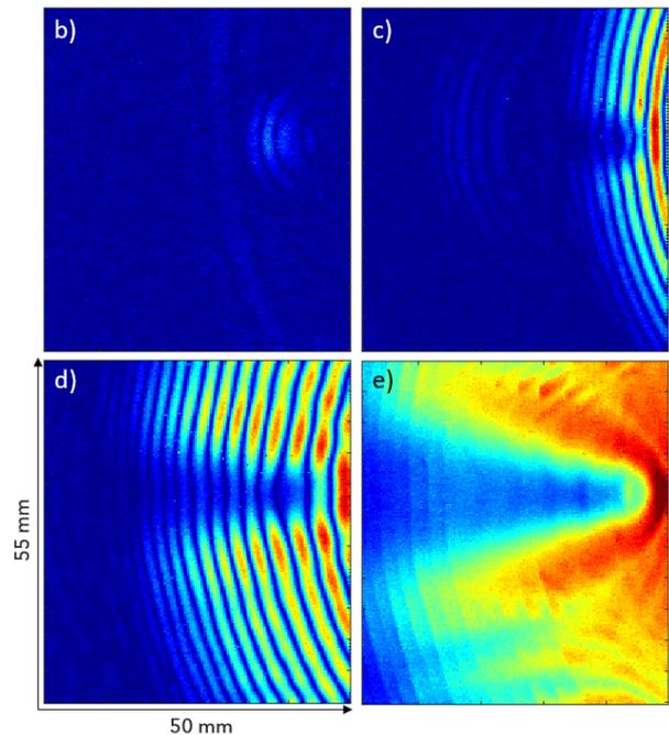
**Figure 5:** Results of the single-sided measurements. (a) Typical time trace showing a guided wave within the first 110  $\mu\text{s}$  and later arrival of an air-coupled signal from the excitation spot. (b)-(d) Time evolution of the guided wave. (b)  $S_0$  wave and  $A_0$  component from the spot weld. (c), (d) diffraction of an  $A_0$  mode around the spot weld. (e) Maximum amplitude projection over 20  $\mu\text{s}$  span showing the amplitude distribution around the weld.
