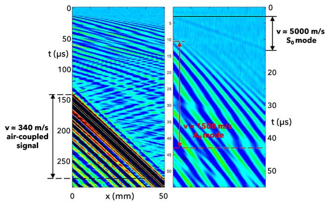
**Figure 6:** B-scan to identify observed modes based on their propagation velocity. The sensor was scanned over a 50 mm distance aligned with the excitation spot. Left panel: 290  $\mu\text{s}$  time segment containing the guided wave as well as the air-coupled signal at late times. Right panel: Zoom to the first 55  $\mu\text{s}$ , allowing the phase velocity estimation for two Lamb modes identified as  $A_0$  and  $S_0$  mode.
