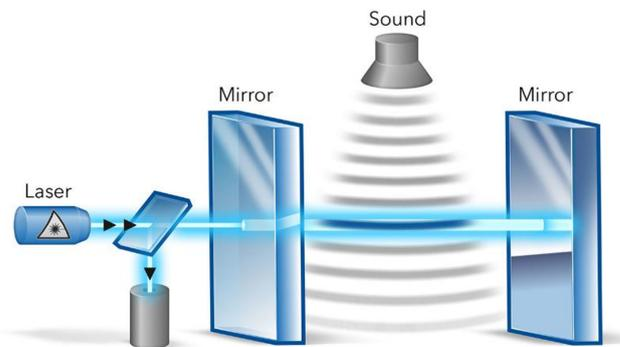
**Figure 1:** Optical microphone: detection principle. The wavelength of light in a medium depends on its refractive index, which is a function of the local density. Since sound modulates the density, it also modulates the optical wavelength, which can be detected with a rigid Fabry-Pérot etalon. The intensity reflected by the etalon depends on the wavelength of the laser in the medium between the mirrors, which is measured with a photodiode.
