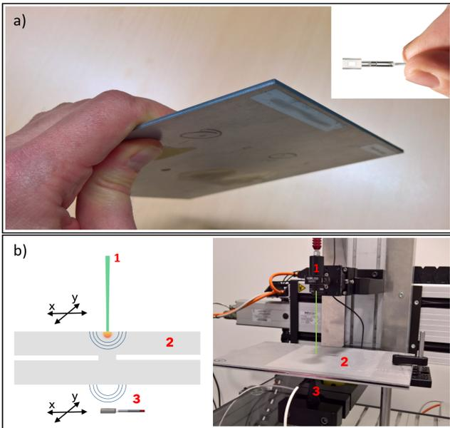
**Figure 2:** Sample used for measurements and detection setup. (a) All measurements have been performed on a spot welding sample consisting of two welded steel plates with dimensions of 20 cm by 20 cm and 1 mm thickness. Inset: optical microphone. (b) Through-transmission detection setup. Left panel: schematics; right panel: actual detection setup. 1: fiber-coupled excitation laser head, 2: sample, 3: optical microphone. Both the laser head and the sample were scanned to generate C-scans.
