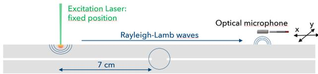
**Figure 4:** Schematics of the single-sided measurement setup. The excitation laser was delivered to a fixed point on the sample at a 7 cm distance to the spot weld. The optical microphone was positioned on the same side of the sample and scanned across a 5 cm by 5.5 cm imaging region containing the spot weld to detect guided waves propagating along the plate.
