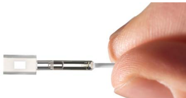
Fig. 1. Function principle of the optical microphone and image of the sensor head. The modulation of the refractive index of air by interaction with sound waves is measured with a rigid Fabry-Pérot interferometer. The mirrors are at the sides of the rectangular opening.
