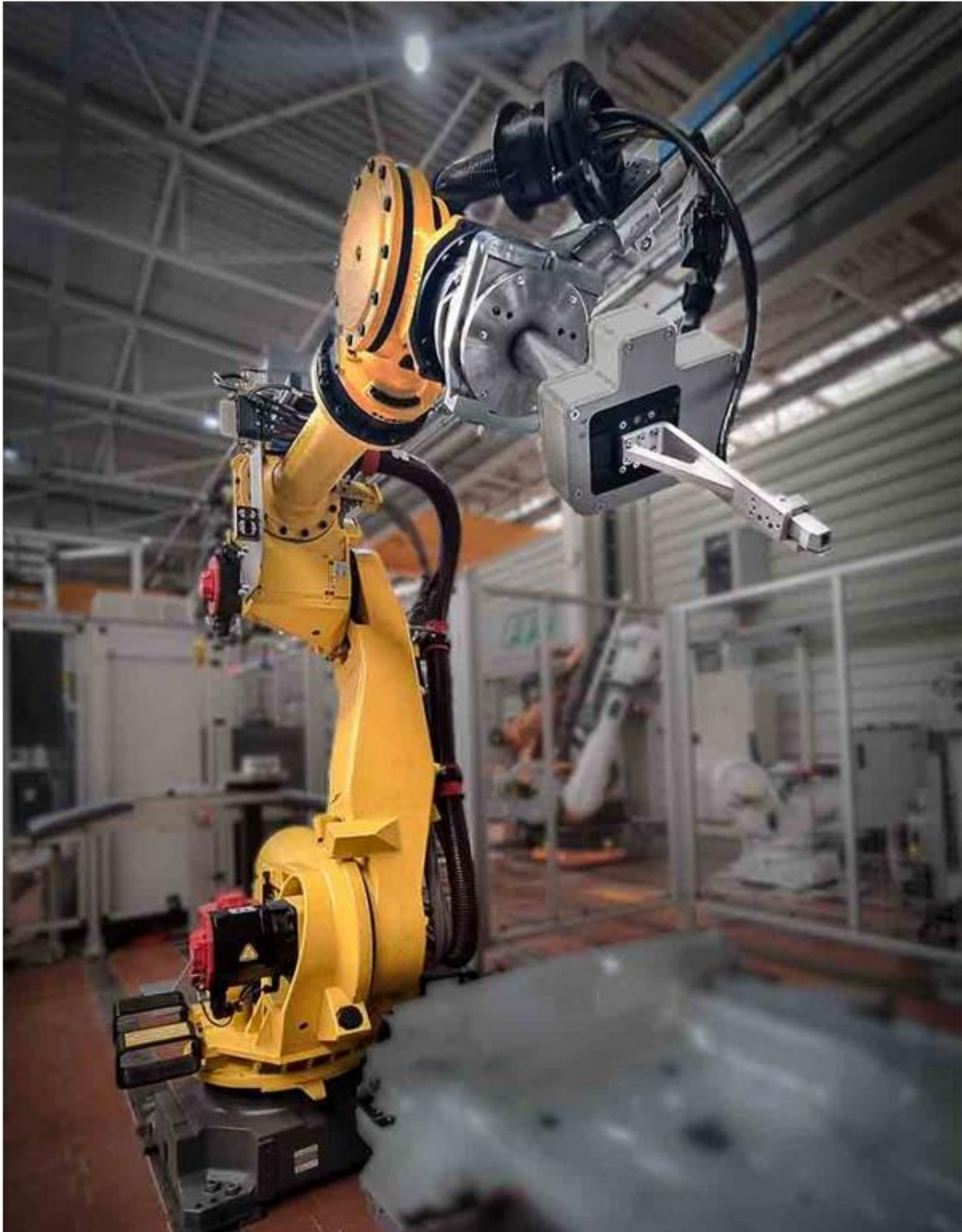
Figure 5: Robot-integrated system for spot-weld inspection. The compact and fiber-coupled probe head for non-contact ultrasonic testing enables straightforward integration. Source: XARION Laser Acoustics GmbH
