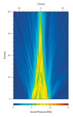
Ultrasound field scan of a piezoelectric emitter with an optical microphone
