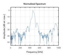
Time signal and normalized spectrum of a piezoelectric emitter measured with the optical microphone
