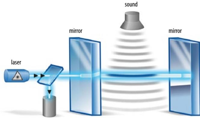
Fig. 2 Principle of operation of the optical microphone. The ultrasonic signal is detected optically by the change of the refractive index within a Fabry-Pérot etalon.
