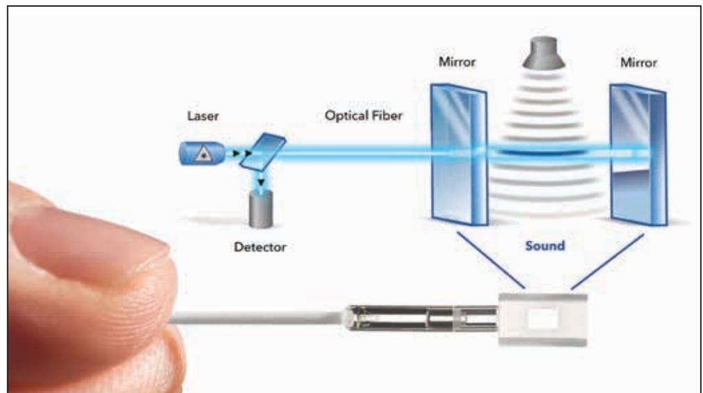
Figure 1 Sensing principle of the optical microphone.
