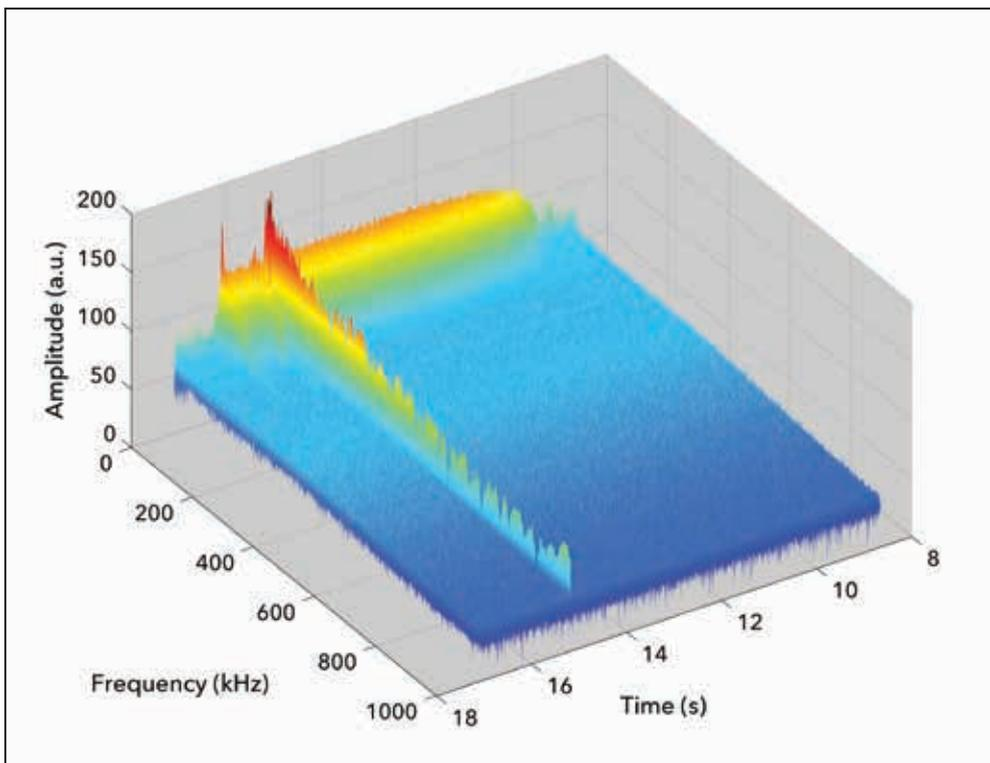
**Figure 3** 3D spectrogram of the sound recorded emitted during the experiment. While the drill noise falls off rapidly above 100 kHz, the fracture of the pencil lead near the 15 sec mark emits an acoustic shock front that spans the entire measurement range.
