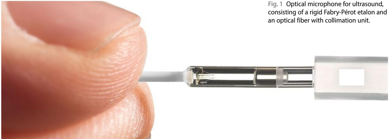
Fig. 1 Optical microphone for ultrasound, consisting of a rigid Fabry-Pérot etalon and an optical fiber with collimation unit.
