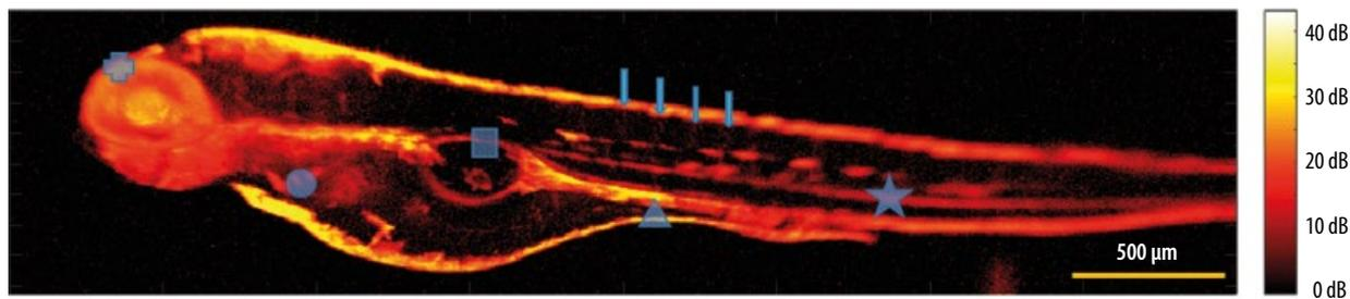
**Fig. 6** Photoacoustic microscopy image using the optical hydrophone, showing a propylthiouracil-treated zebrafish larva, 120 hours after fertilization. The color bar indicates the SNR in decibels. Blue arrows: intersegmental vessels; blue square: swim bladder; blue cross: eye; blue circle: heart; blue star: dorsal aorta; tip of blue triangle: axial vein. Figure taken and adapted from [5].
